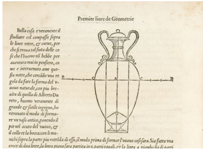
Both Dürer and Serlio introduce the principle of drawing arcs taking the ovum as an example. The construction begins with the divisions of an orthogonal frame. The radii measurements are based on the approximations of the harmonic section.
